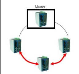
If the number of Ethernet switches in the Turbo Ring is 2N (an even number), the backup segment is one of the two segments connected to the (N+1)st switch (i.e., the unit directly opposite the master).
